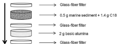
Figure 3. Scheme of a filled extraction cell for SPLE [6,7]
